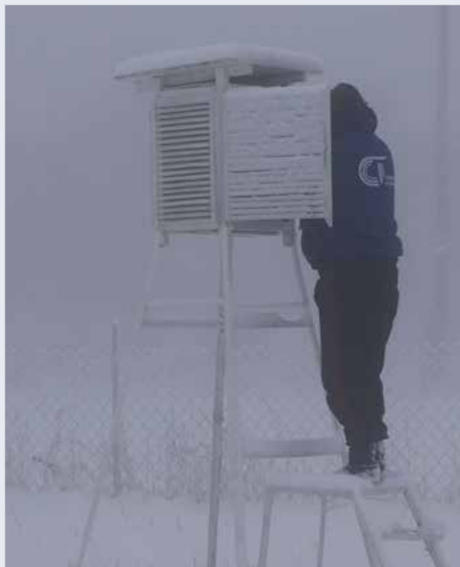
Kyrgyzhydromet specialist maintaining manual equipment under extreme climate conditions. Source: U. Torobekov, 2016.
