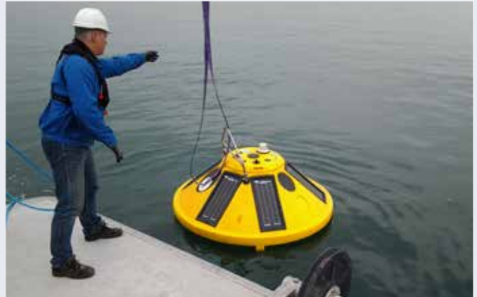
Commissioning of a oceanographic monitoring buoy in the Gulf of Trieste, Adriatic Sea. Source: L. Ravnik, ARSO, 2014.
