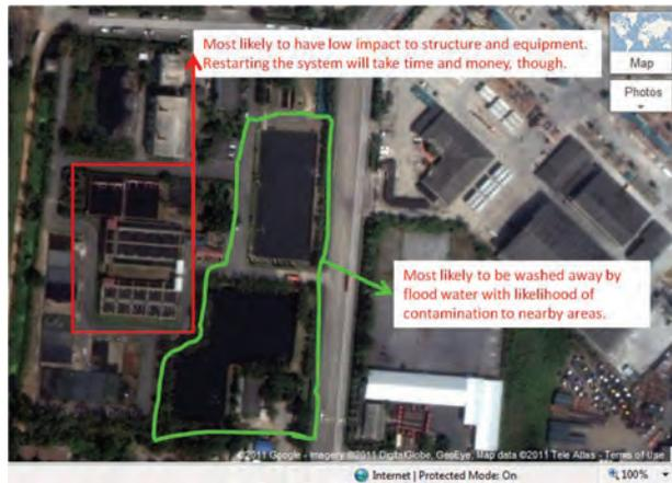
cubic-meters of water per day. Figure 19: Waste water treatment facility plant illustrates the Bang Pa-in Industrial Estate before the flood and the potential impacts of flooding. Normally the treatment structure can withstand minor flooding, however, certain equipment, the control system and the piping structure are vulnerable to heavy floods. Furthermore, finishing ponds or open lagoons are typically built at ground level,
