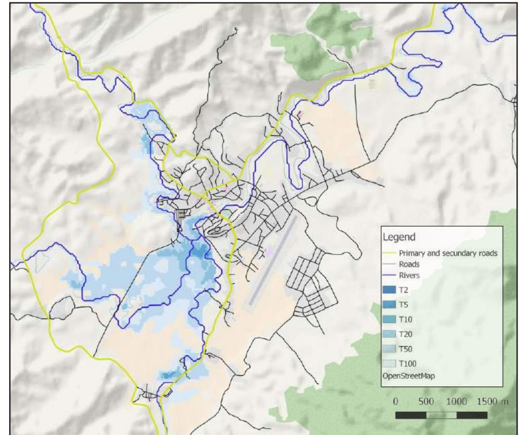
Fig. 6.9 Simulated flood extent after implementing all four measures (river improvements, schorcut, dikes and reservoirs) compared to the reference case (flood event of August 2008) (Source: Deltares, 2017)
