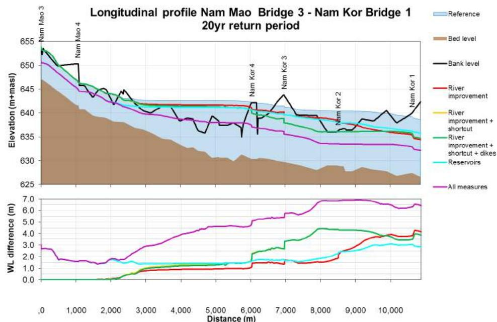
Fig. 6.11 Longitudinal profile showing the decrease in water levels resulting from the implementation of all four measures for a 20-year return period. (Source: Deltares, 2017)
