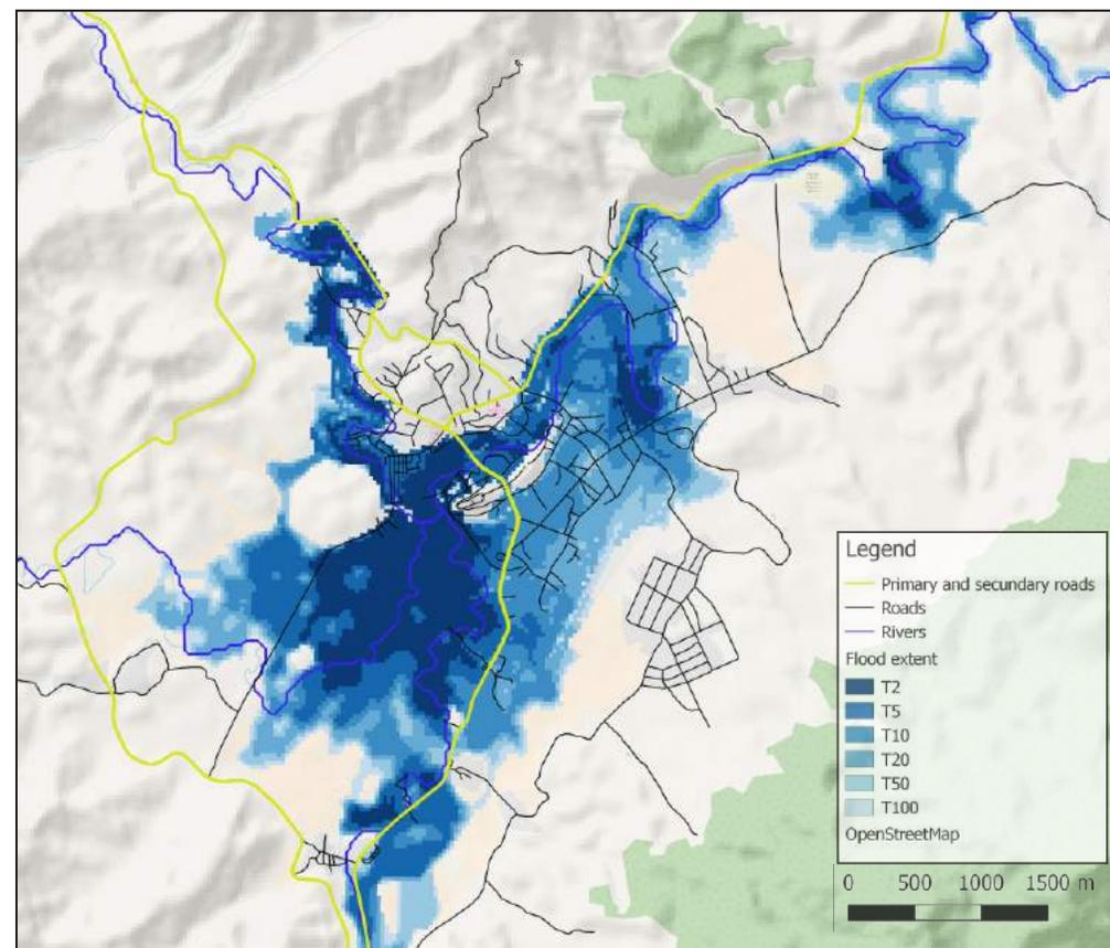
Figure 3.3 Flood extent for the reference case, flood event of August 2008. (WFLOW; Manning's coefficient,  $n = 0.045 \text{ s/m}^{1/3}$ ) (Source: Deltares 2017)
