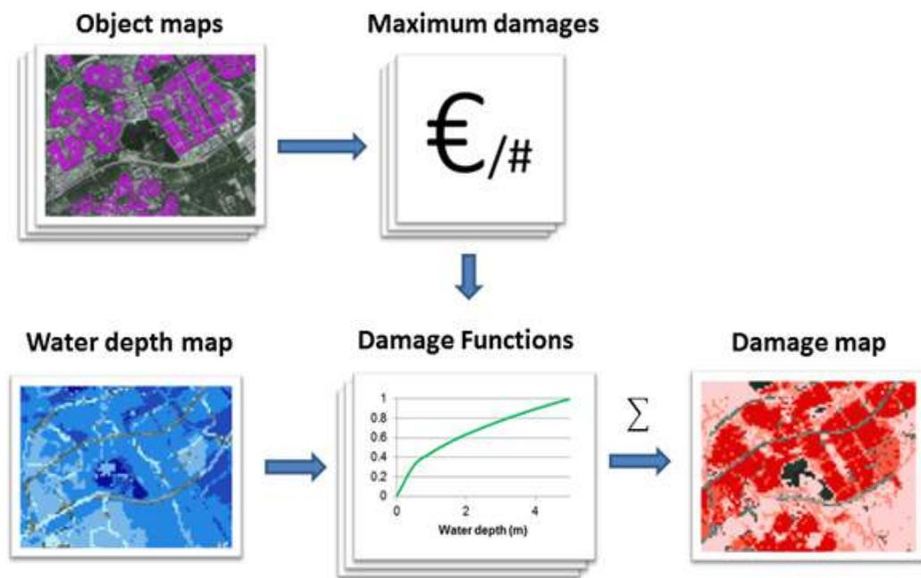
Figure 3.4 Overview of the damage calculation
