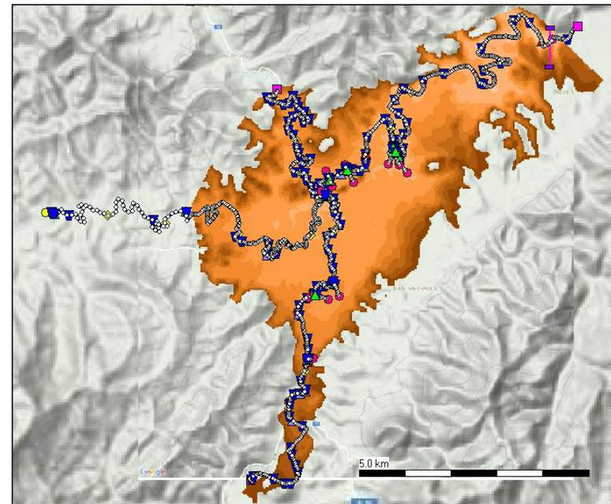
Fig. 3.2 Overview of 1D2D hydraulic model built in SOBEK.
