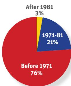
**Figure 8.** Percentage of buildings collapsing in Kobe earthquake, by construction date
