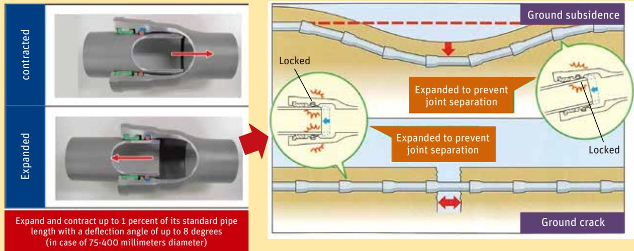
Source: ©Japan Ductile Iron Pipe Association. Reproduced, with permission, from Japan Ductile Iron Pipe Association; further permission required for reuse.
