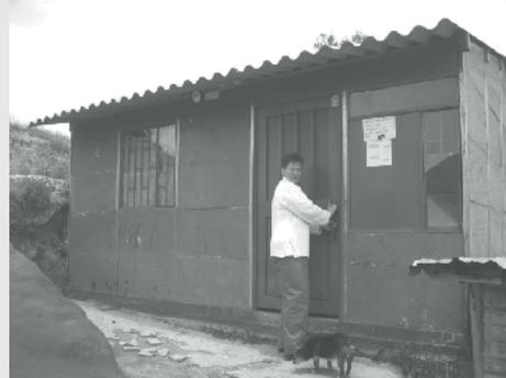
**SIMPLE MASONRY HOUSES**—5 percent of the total. These are typically built with trussed stonework without a structure (to attach to), cyclops foundations, and a foundation beam to support possible add-ons.
