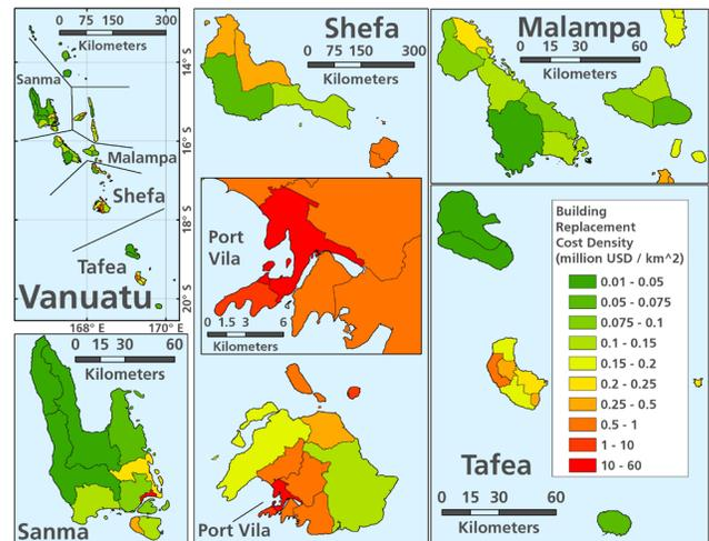
Figure 2: Building replacement cost density by village.
