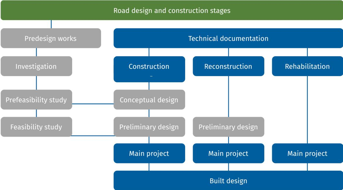
Note: Grey boxes indicate stages that use engineering geological mapping for geohazard risk evaluation. Blue boxes indicate design stages that assess simple geohazard risk evaluation within engineering geological mapping.
