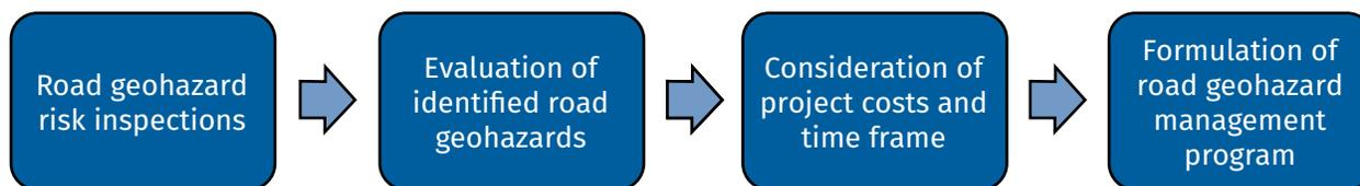
The MLIT’s Road Bureau can request thematic subnational and nationwide inspections (such as tunnel portal slope inspections in 1996 and the inspections of large roadside rock-mass slopes in 1997) from the abovementioned road management authorities.
