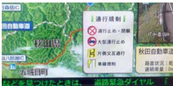
The legend at the bottom of the screen helps viewers to identify road traffic situations: whole-width closures, partial-width closures, closures for large vehicles only, or road subsections with alternating one-way traffic.
