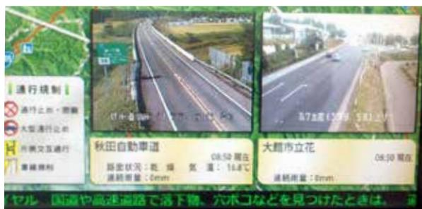
The information board displays closed-circuit television (CCTV) monitoring images of hazard-prone road locations with weather conditions such as temperature and cumulative rainfall amount from the start of the rainfall.
