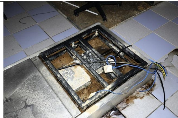
Figure 2: Though cleaned up externally, penetration of water and soil destroyed this and all other luggage scales.
