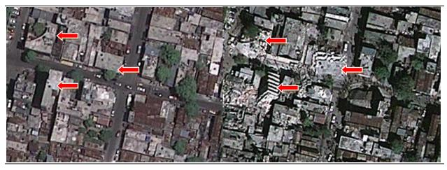
Figure 6.5 Pre- (left) and Post-event (right) Imagery of "Pancaked" and "Stair-step" Damage Patterns
