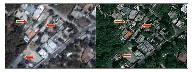
Figure 6.6 Pre- (left) and Post-event (right) Imagery displaying examples of Recent Construction and Structures without Roofs
