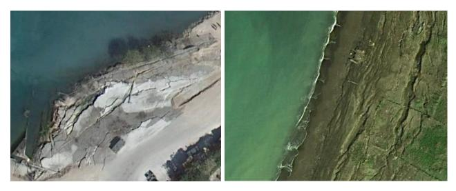
(d) Ground cracking is readily apparent parallel to the coastline (both left and right images show ground cracking)
