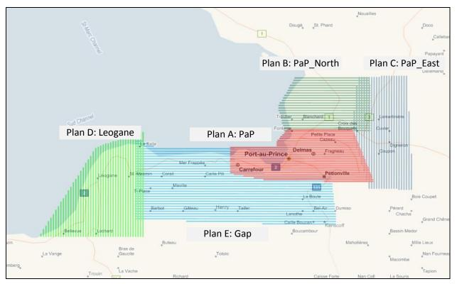
Figure 2.2 Flight Plans Apportioned into Five 1-Day Coverage Areas
