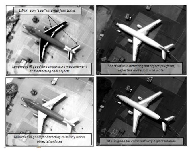
Figure 4.2 Four Cameras for Color and Infrared Imaging
