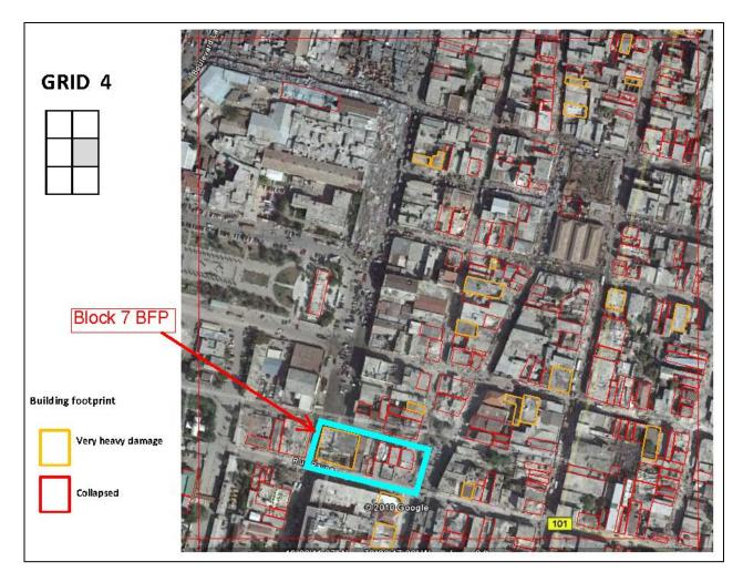
Figure 6.11 Plan View of Damage Assignments Completed by BFP for Central PaP (Fierro, 2010)
