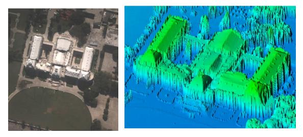
Figure 10.1 The National Palace as viewed in Optical Imagery (left) and LiDAR
