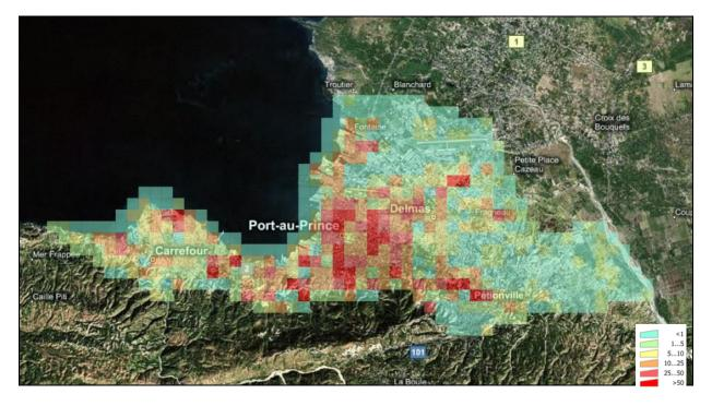
Figure 8.2(a) Number of Collapsed Buildings pejur 500 m Grid Cell
