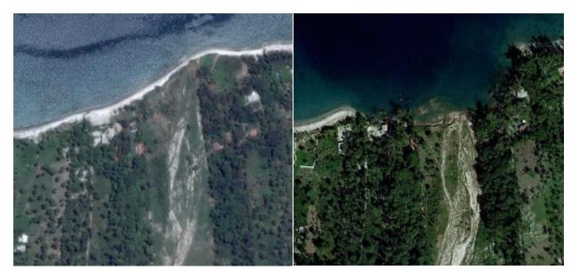
(c) For coastal slumping, it is most useful to compare pre- (left image) and post-event (right image) shorelines. Coastal slumping will show significant coastal retreat and loss of beach zone.
