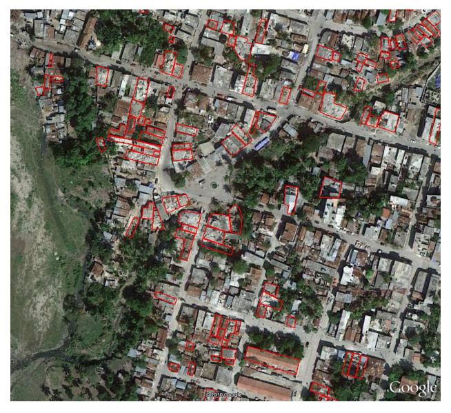
Figure 8.7 Locations of Collapsed and Heavily-Damaged Buildings in Jacmel (Footprints in Red)
