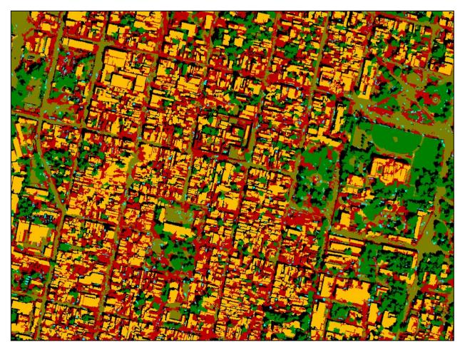
Figure 10.7 Identification of Building Footprints along with Rubble and Debris Areas for Downtown Port-au-Prince
