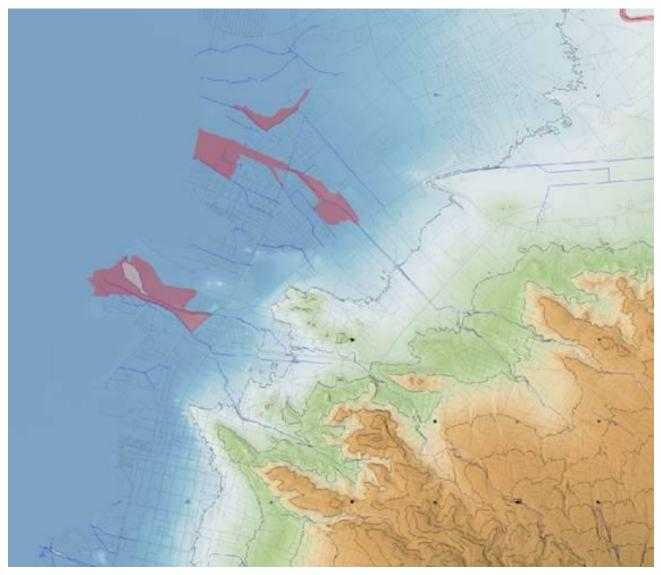
Figure 10.5 Ground Elevation GIS Layer with Flood Areas Mapped in Red (WB-IC-RIT LiDAR Data; Corps of Engineers)
