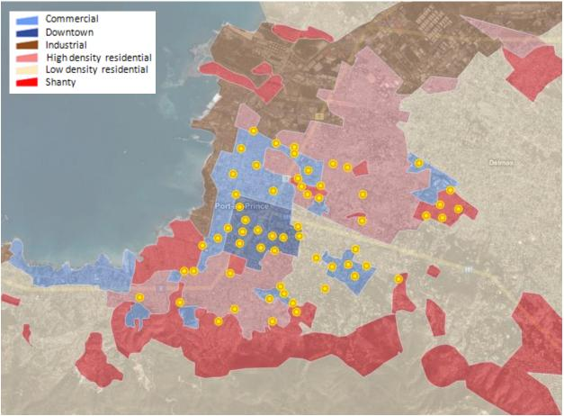
Figure 8.9 CAR Damage Survey Locations (60 total shown in yellow) in Port-au-Prince, Overlaid on Land-use Map
