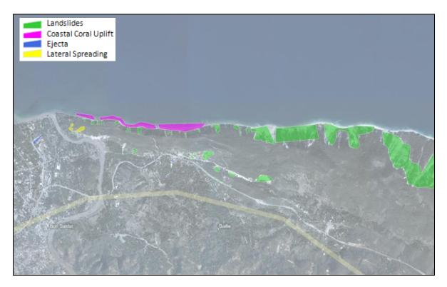
Figure 6.16 Liquefaction Assessment Data Layer - available for download via the VDV site
