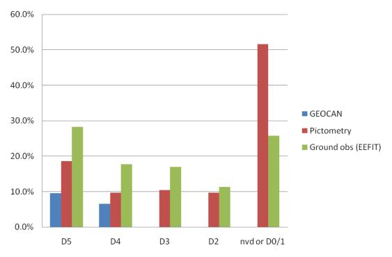
Figure 8.12 Comparison of GEO-CAN, Pictometry and EEFIT Damage Results. Sample size = 124
