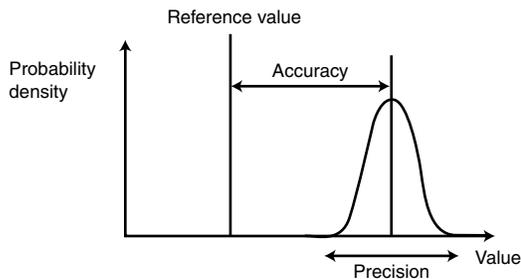
Precision (stability) of a measure vs. accuracy (conformity to actual value).
