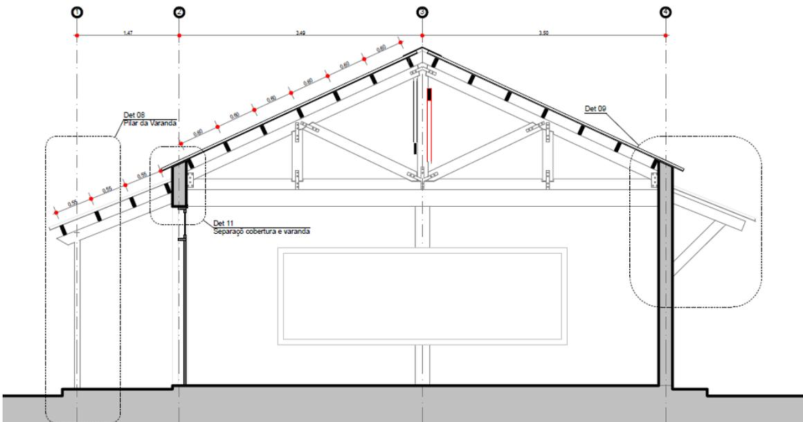
Figure 5.4 Sketch for placing pillars to support roof extension (from UN-Habitat, 2015)
