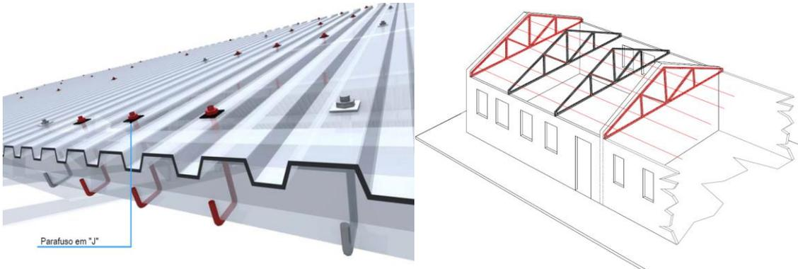
Figure 5.3 Sketch for improving connection between wall, frame and roof (from UN-Habitat, 2015)
