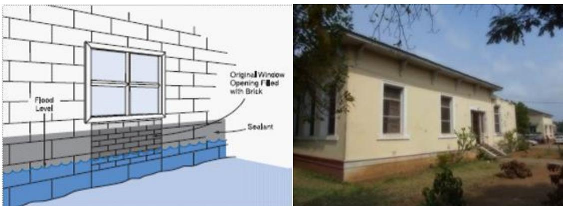
Figure 5.1 Sketch for dry flood proofing and local example of Xai Xai
