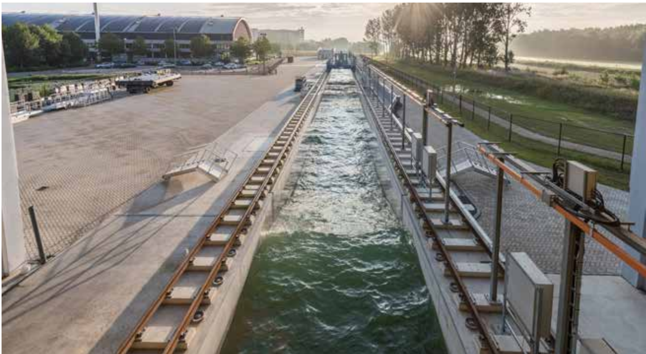
Experimental facilities such as this Delta Flume can be used to test vegetation performance under extreme conditions
