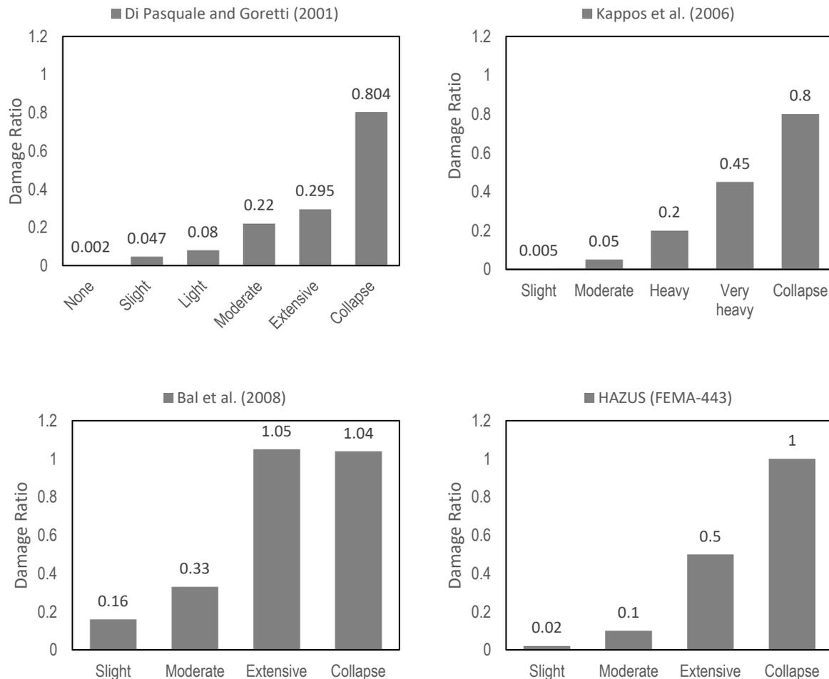
**Figure 4. Comparison of the suggested consequence function mean damage ratios by Di Pasquale and Goretti (2001), Kappos et al. (2006), Bal et al. (2008) and HAZUS (FEMA 2003).**
