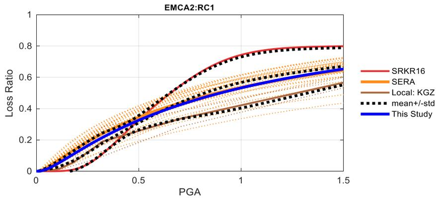
Figure 13. Comparison between the vulnerability functions of different studies for residential building class EMCA2: RC1. Note: the thin dotted lines represent the individual study of a group while the thicker solid lines show the mean of the group. The same colour was used for both in the figure. The blue line shows the parametric vulnerability function before calibration.
