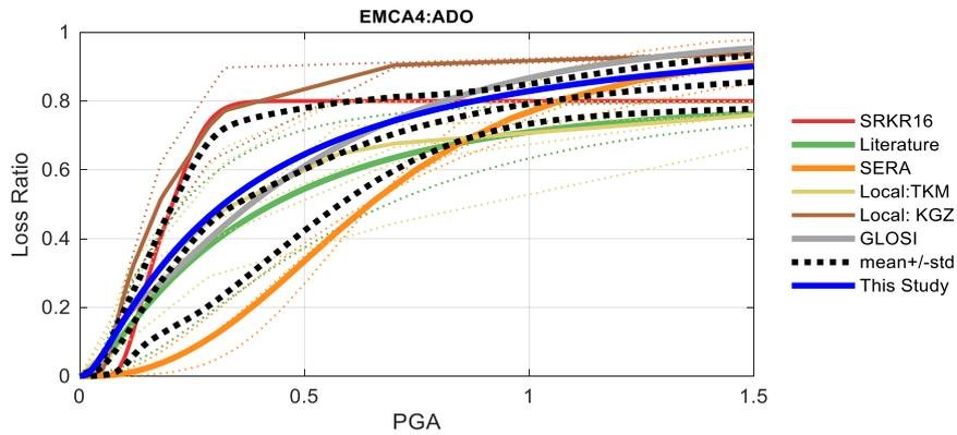
Figure 19. Comparison between the vulnerability functions of different studies for residential building class EMCA4: ADO. Note: the thin dotted lines represent the individual study of a group while the thicker solid lines show the mean of the group. The same colour was used for both in the figure. The blue line shows the parametric vulnerability function before calibration.
