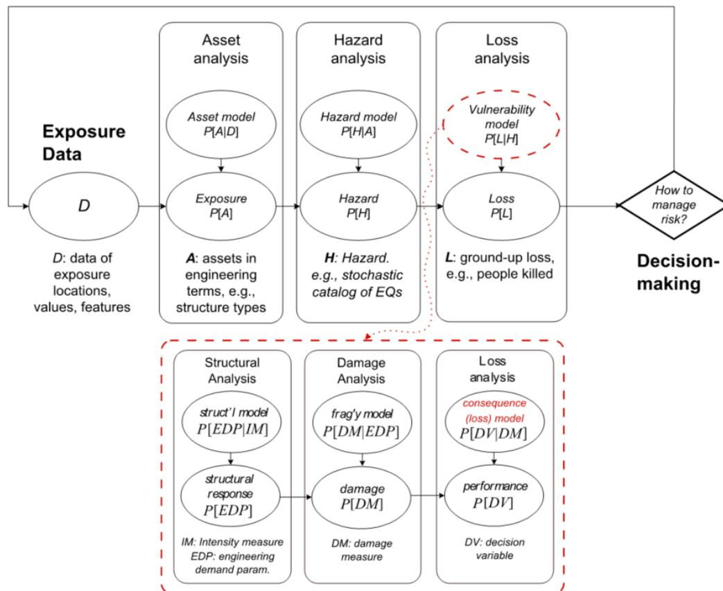
Figure 1. Conceptual workflow of a risk analysis procedure. Upper row illustrates the three major analysis components, while the bottom row provides a zoomed view of the sub-components of analytical (which is very often adopted) vulnerability modelling stage.
