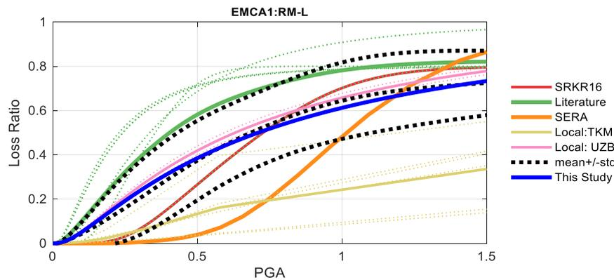
Figure 11. Comparison between the vulnerability functions of different studies for residential building class EMCA1: RM-L. *Note: the thin dotted lines represent the individual study of a group while the thicker solid lines show the mean of the group. The same colour was used for both in the figure. The blue line shows the parametric vulnerability function before calibration.*
