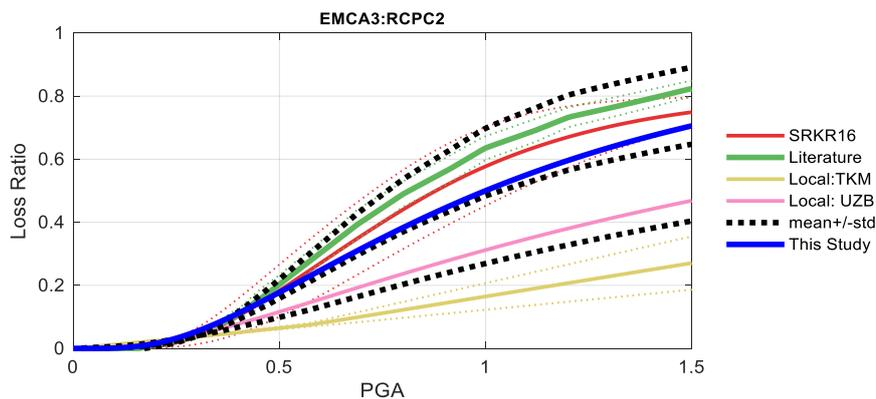
Figure 18. Comparison between the vulnerability functions of different studies for residential building class EMCA3: RCPC2. Note: the thin dotted lines represent the individual study of a group while the thicker solid lines show the mean of the group. The same colour was used for both in the figure. The blue line shows the parametric vulnerability function before calibration.
