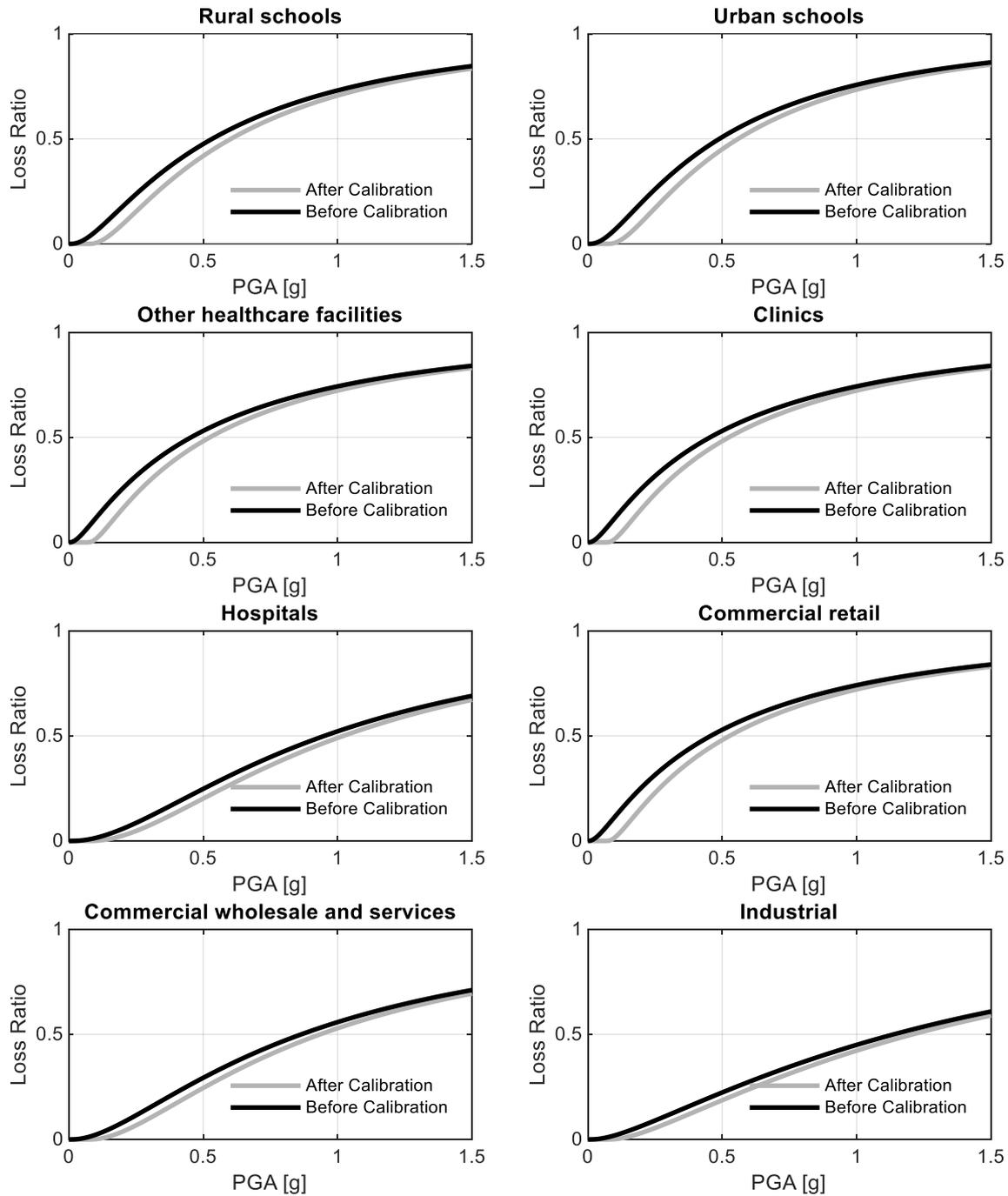
Figure 26. Comparison between the proposed vulnerability functions among different classes of the non-residential buildings before and after calibration.
