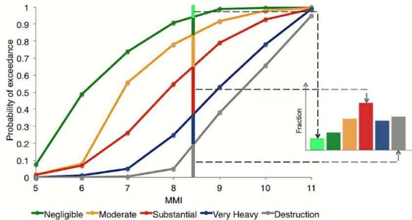
Figure 3. Schematic illustration of combining global fragility functions and associated consequence function. In this example the IM is expressed in terms of Modified Mercalli Intensity.
