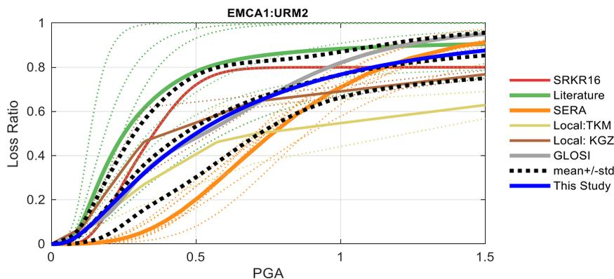
Figure 9. Comparison between the vulnerability functions of different studies for residential building class EMCA2: URM2. Note: the thin dotted lines represent the individual study of a group while the thicker solid lines show the mean of the group. The same colour was used for both in the figure. The blue line shows the parametric vulnerability function before calibration.
