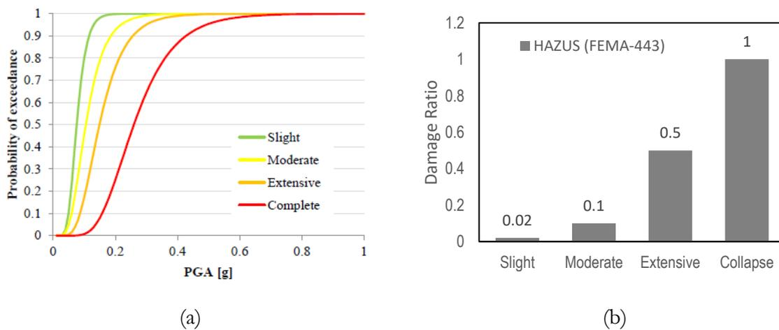
Figure 2. (a) An example of Fragility Functions for four global damage states (slight, moderate, extensive and collapse) as a function of PGA as the ground motion IM for a hypothetical building; (b) An example of consequence function linked to the global fragility curves.
