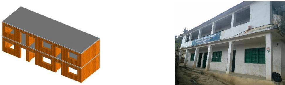
Figure 7. Rectangular block in Cement Mortar Masonry (UCM-URM 7 mid-rise with low seismic design)-GLOSI
