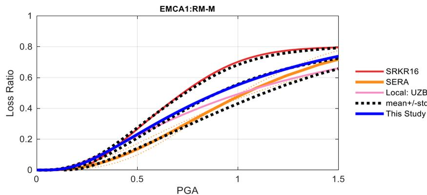
Figure 12. Comparison between the vulnerability functions of different studies for residential building class EMCA1: RM-M. *Note: the thin dotted lines represent the individual study of a group while the thicker solid lines show the mean of the group. The same colour was used for both in the figure. The blue line shows the parametric vulnerability function before calibration.*
