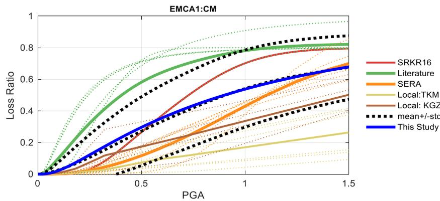
Figure 10. Comparison between the vulnerability functions of different studies for residential building class EMCA1: CM. *Note: the thin dotted lines represent the individual study of a group while the thicker solid lines show the mean of the group. The same colour was used for both in the figure. The blue line shows the parametric vulnerability function before calibration.*
