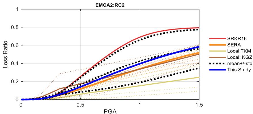
Figure 14. Comparison between the vulnerability functions of different studies for residential building class EMCA2: RC2. Note: the thin dotted lines represent the individual study of a group while the thicker solid lines show the mean of the group. The same colour was used for both in the figure. The blue line shows the parametric vulnerability function before calibration.
