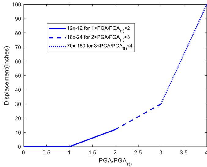
**Figure 27. Lateral spreading displacement relationship- HAZUS**
