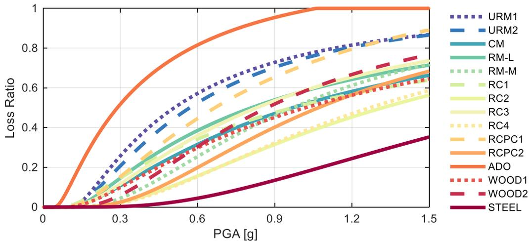
Figure 23. Comparison of the proposed vulnerability functions for different classes of residential buildings after calibration
