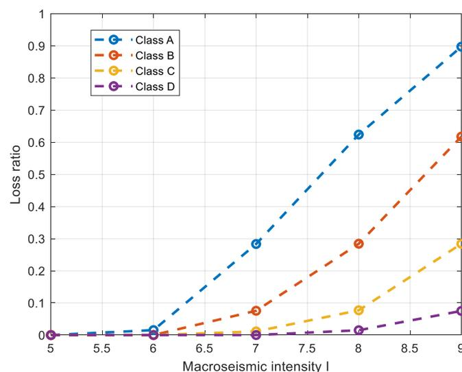
Figure 5. Vulnerability curves-Kyrgyz Republic provided by the local partners. Legend: different lines in the figure refer to the different classes of A, B, C and D. Note: The curve for class E was almost always zero for the range of intensities considered in the plot and hence was discarded for improving clarity of the chart.
