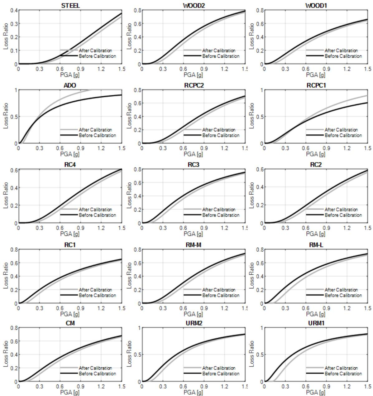
Figure 24. Comparison of the proposed vulnerability functions before and after calibration for different classes of residential buildings.
