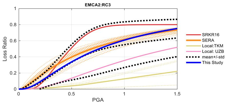
Figure 15. Comparison between the vulnerability functions of different studies for residential building class EMCA2: RC3. Note: the thin dotted lines represent the individual study of a group while the thicker solid lines show the mean of the group. The same colour was used for both in the figure. The blue line shows the parametric vulnerability function before calibration.
