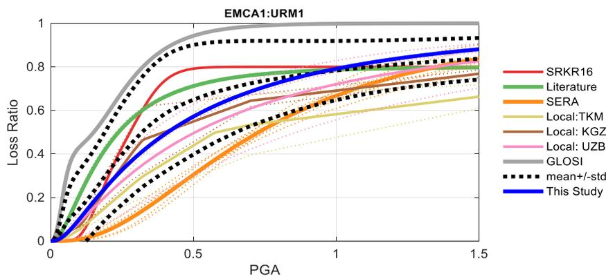
Figure 8. Comparison between the vulnerability functions of different studies for residential building class EMCA1: URM1. Note: the thin dotted lines represent the individual study of a group while the thicker solid lines show the mean of the group. The same colour was used for both in the figure. The blue line shows the parametric vulnerability function before calibration.
