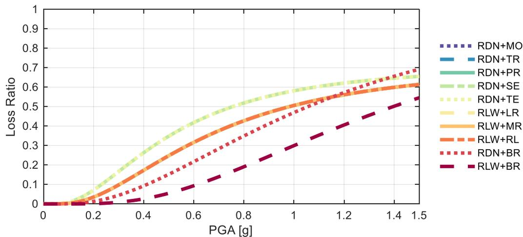
**Figure 28.** Comparison between different vulnerability functions considered for the infrastructure. The chart includes two groups of coincident curves: Group 1='RDN+MO', 'RDN+TR', 'RDN+PR', 'RLW+LR', 'RLW+MR', and 'RLW+RL' and Group 2='RDN+SE' and 'RDN+TE' that have the same vulnerability curve as discussed above.
