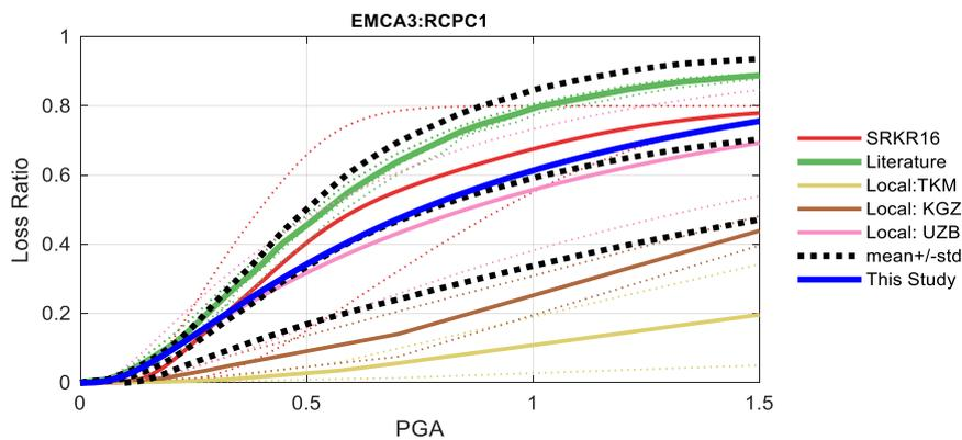
Figure 17. Comparison between the vulnerability functions of different studies for residential building class EMCA3: RCPC1. Note: the thin dotted lines represent the individual study of a group while the thicker solid lines show the mean of the group. The same colour was used for both in the figure. The blue line shows the parametric vulnerability function before calibration.
