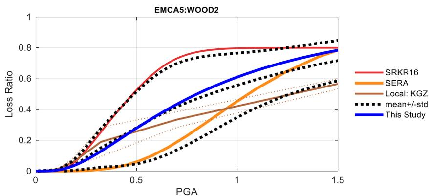
Figure 21. Comparison between the vulnerability functions of different studies for residential building class EMCA5: WOOD2. Note: the thin dotted lines represent the individual study of a group while the thicker solid lines show the mean of the group. The same colour was used for both in the figure. The blue line shows the parametric vulnerability function before calibration.
