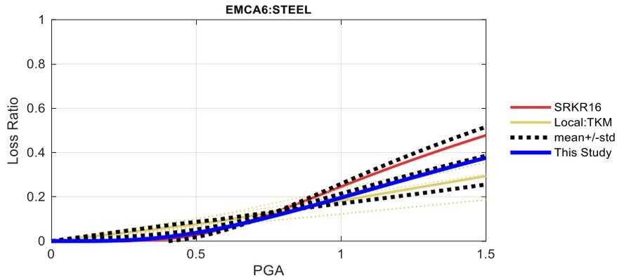
Figure 22. Comparison between the vulnerability functions of different studies for residential building class EMCA5: STEEL. *Note: the thin dotted lines represent the individual study of a group while the thicker solid lines show the mean of the group. The same colour was used for both in the figure. The blue line shows the parametric vulnerability function before calibration.*
