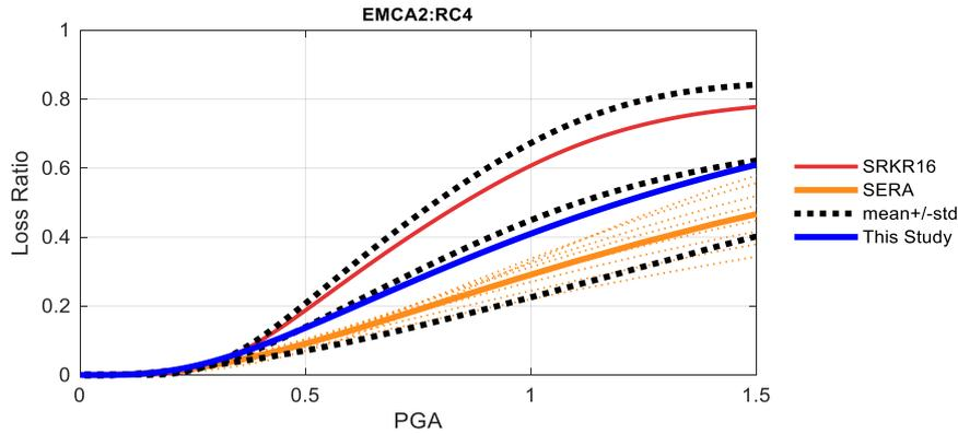
Figure 16. Comparison between the vulnerability functions of different studies for residential building class EMCA2: RC4. Note: the thin dotted lines represent the individual study of a group while the thicker solid lines show the mean of the group. The same colour was used for both in the figure. The blue line shows the parametric vulnerability function before calibration.
