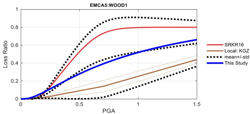
Figure 20. Comparison between the vulnerability functions of different studies for residential building class EMCA5: WOOD1. Note: the thin dotted lines represent the individual study of a group while the thicker solid lines show the mean of the group. The same colour was used for both in the figure. The blue line shows the parametric vulnerability function before calibration.
