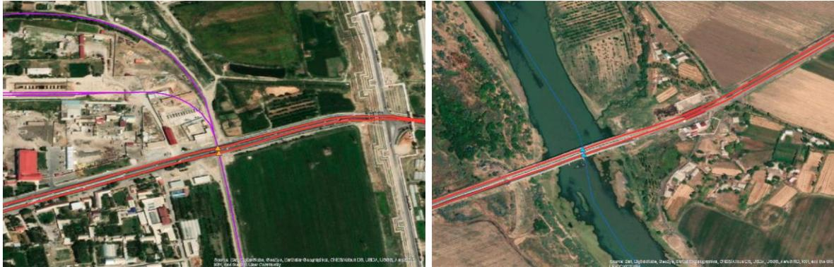
Figure 30. Left: Railway and road segments (purple and red lines, respectively) extracted from OSM. The yellow triangles locate a bridge identified by the consortium in the intersection between main transport infrastructures. Right: Example of bridge identified by intersecting the highway/motorway/trunk road network with the main rivers.
