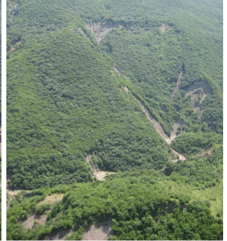
Photo E. 12. Unloaded soil slips illustrating possibility of collapse and subsequent damming of the Vere River
