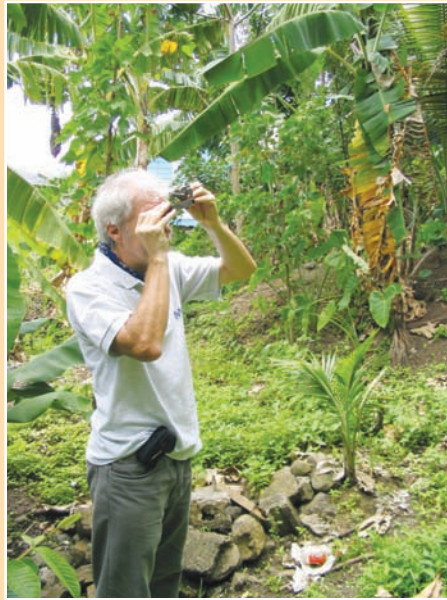
b. Abney level being used to measure slope angle.
