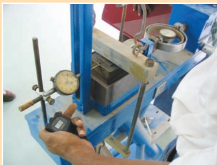
FIGURE 3.20 Shear box used to determine soil strength parameters
