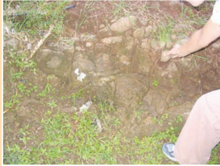
a. Grade II material transitioning to Grade III above.
