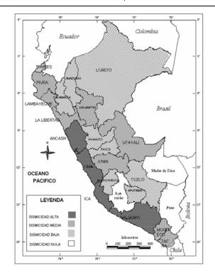
Figure 1. Seismic Hazard Map of Peru.
