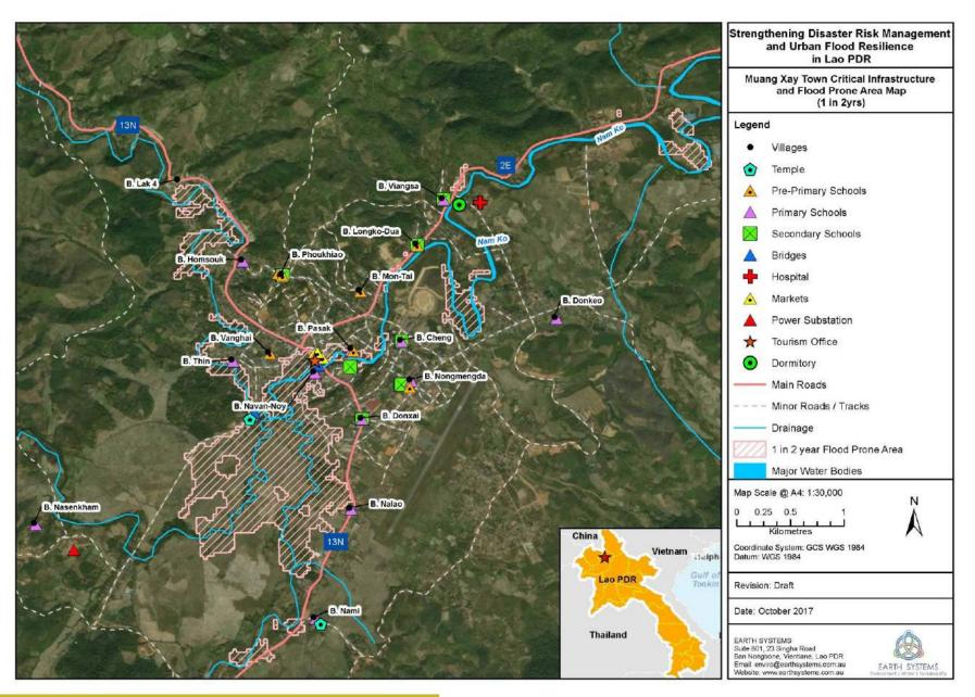
Fig. 4.5 *Critical infrastructure and expected flood prone area for a 1 in 2-year flood event (Source: Earth Systems, 2017)*
