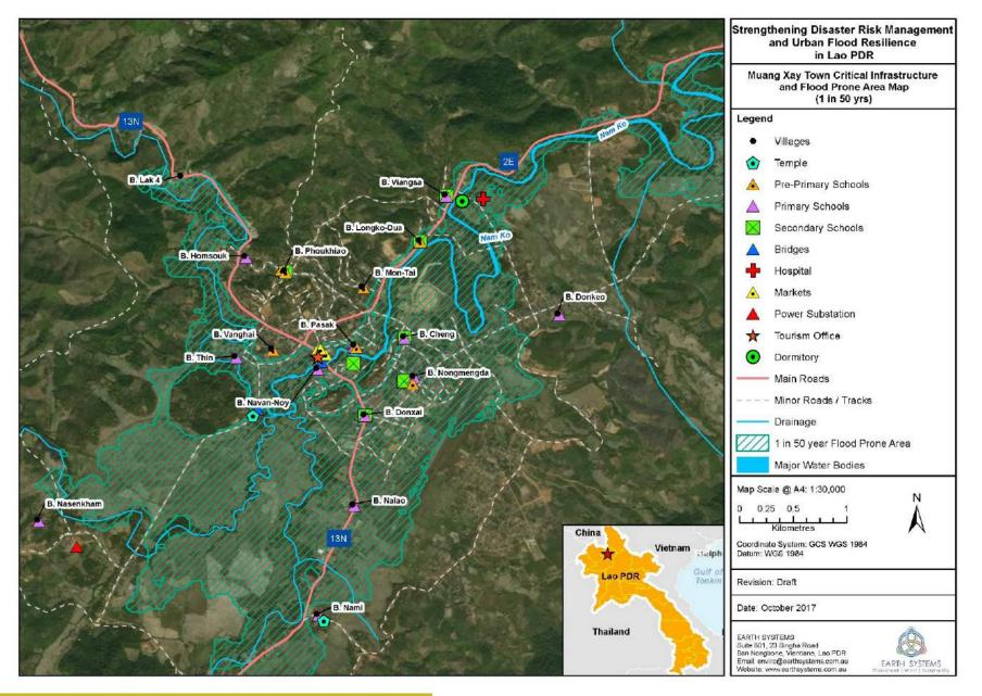
Fig. 4.9 *Critical infrastructure and expected flood prone area for a 1 in 50-year flood event (Source: Earth Systems, 2017)*
