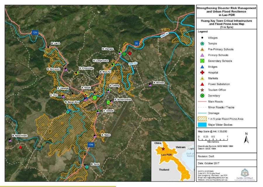
Fig. 4.6 *Critical infrastructure and expected flood prone area for a 1 in 5-year flood event (Source: Earth Systems, 2017)*
