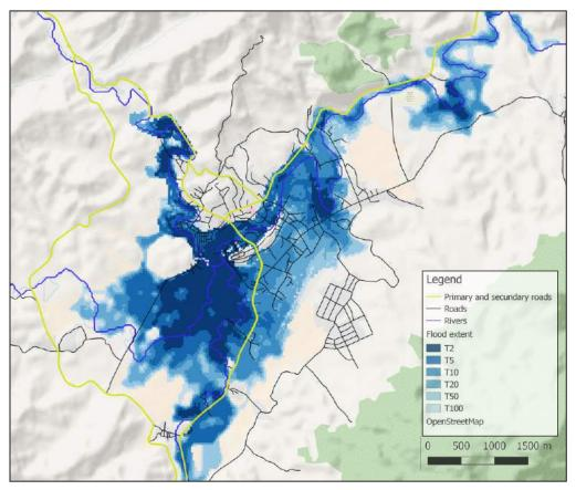
Figure 3.3 Flood extent for the reference case, flood event of August 2008. (WFLOW; Manning's coefficient, n = 0.045 s/m1/3) (Source: Deltares 2017)
