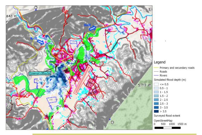
Fig. 4.3 Overlay of the simulated flood map of the September 2008 event on the surveyed flood extent (green area). The overlay of this simulated flood extent and the survey show a good fit in some parts of the Muang Xay area. However, and as expected in some areas (e.g. near the future river park) there is only a limited fit. Given the available data, the simulation results are considered as acceptable.
