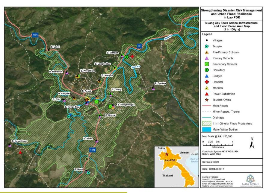
Fig. 4.10 *Critical infrastructure and expected flood prone area for a 1 in 100-year flood event (Source: Earth Systems, 2017)*
