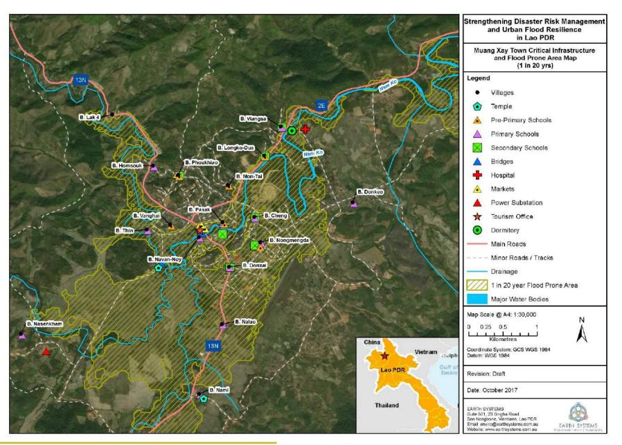
Fig. 4.8 *Critical infrastructure and expected flood prone area for a 1 in 20-year flood event (Source: Earth Systems, 2017)*
