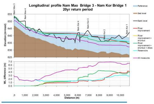
Fig. 6.11 Longitudinal profile showing the decrease in water levels resulting from the implementation of all four measures for a 20-year return period. (Source: Deltares, 2017)
