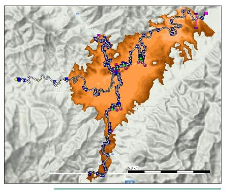
Fig. 3.2 Overview of 1D2D hydraulic model built in SOBEK. (Source: Deltares, 2017)
