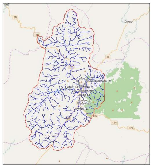
Fig. 3.1 Overview of Hydrological model. Muang Xay Rivers and streams as applied in WFLOW. The grey dots represent the lateral connections. (Source: Deltares, 2017)
