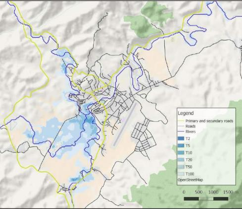
Fig. 6.9 Simulated flood extent after implementing all four measures (river improvements, schorcut, dikes and reservoirs) compared to the reference case (flood event of August 2008) (Source: Deltares, 2017)
