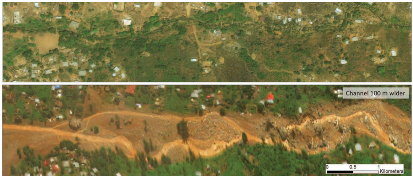
FIGURE 12: Pre- and Post-Disaster Satellite Imagery Showing the Widening of River Channel Downstream
