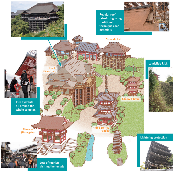
KIYOMIZU-DERA TEMPLE DISASTER PREVENTION MEASURES, THE WORLD BANK DRM HUB
