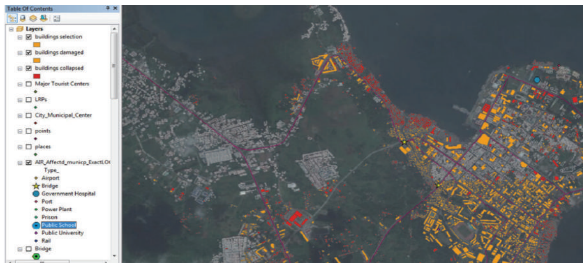
Figure 1.3 Sample Remote Damage Assessment in Tacloban
