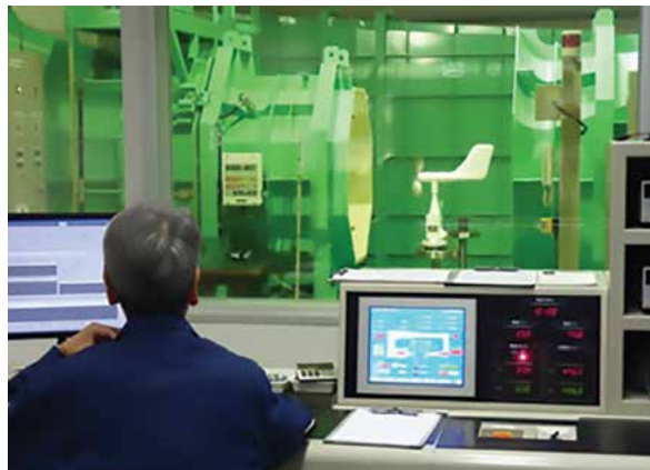
Photo 4.1: Real-time Data Dissemination Operation at JMBSC (left) and Verification of a Wind Vane/Anemometer at the Meteorological Instrument Center (MIC)/JMA by JMBSC Expert (right).
