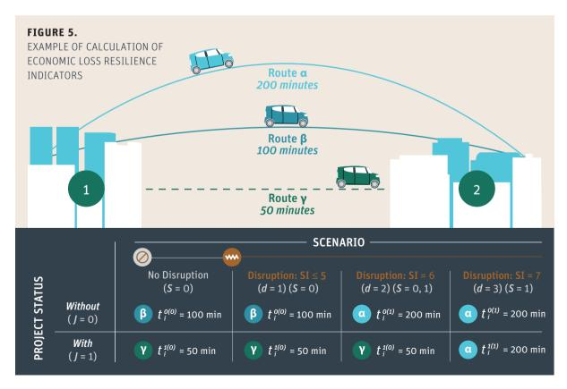
The functionality of the road network will result from the combination between project status (j=0|1) and disruption scenario (d=1|2|3). The travel time of a representative O-D pair is the minimum travel time the available routes. The travel times with and without the project Route  $\gamma$  with no disruption and the three hazard scenarios are as follows:
