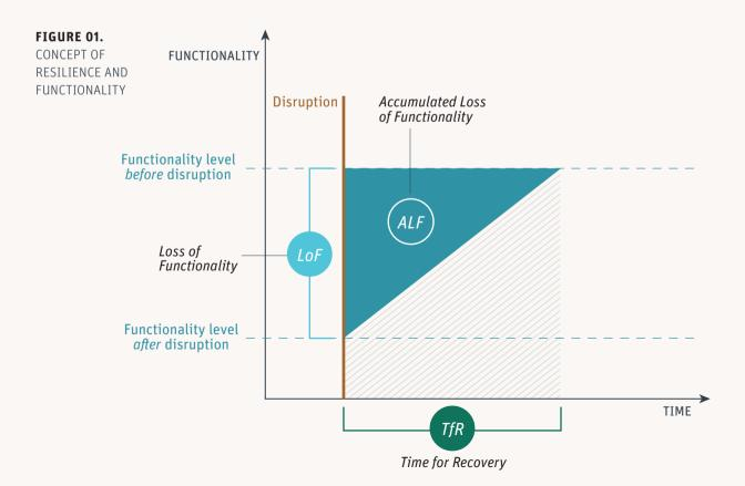
this process. In the event of a disaster, an asset (e.g., a road or bridge) is susceptible to *loss of functionality* (*LoF* •) measured in terms of four dimensions (k): travel time (t), road utilization (u), provision of relief (p) and access to lifesaving services (l).
