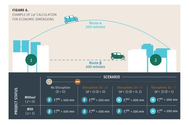
between the O-D pair doubles if scenario 2 occurs in the without-project case, whereas no change in travel time would occur in the with-case since the proposed project would withstand a level 6 earthquake. Given scenario 2, then, *LoF* (the economic loss due to the increase of travel time) arises in the without-project case, but does not in the with-project case. This *LoF* savings over the period of recovery would account for the project's contribution to resilience.
