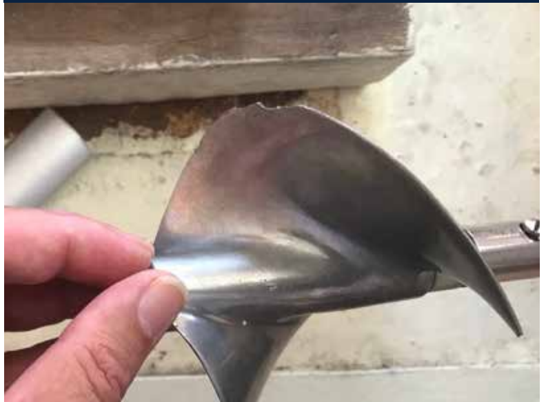
PHOTO 13. PROPELLER OF A CURRENT METER WITH SIGNIFICANT WEAR AND TEAR
