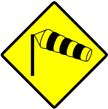
b. Sign code 214: Crosswind caution
