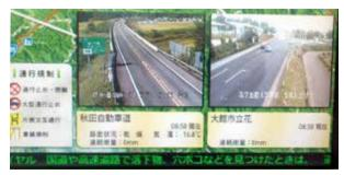
The information board displays closed-circuit television (CCTV) monitoring images of hazard-prone road locations with weather conditions such as temperature and cumulative rainfall amount from the start of the rainfall.
