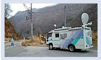
Even if communication lines are disrupted because of a disaster, disaster communication vehicles ensure the continuation of telephone communication, video distribution, and other transmissions in the field using communications satellites. This vehicle was stationed in in Hakuba-mura, Nagano Prefecture, after the North Nagano Prefecture Earthquake in November 2014.
