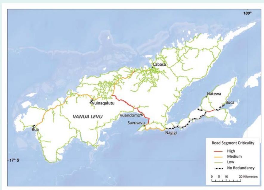
FIGURE B3.1.1: Critical road segments in Viti Levu (right) and Vanua Levu (left). Criticality is measured by the increased road user cost when the road segment is removed from the network.
