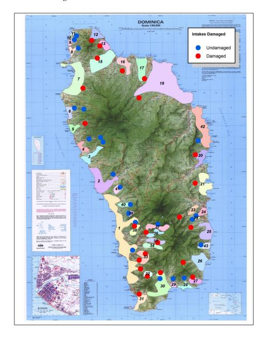
Figure 6 - DOWASCO Service Areas and Intake Status
