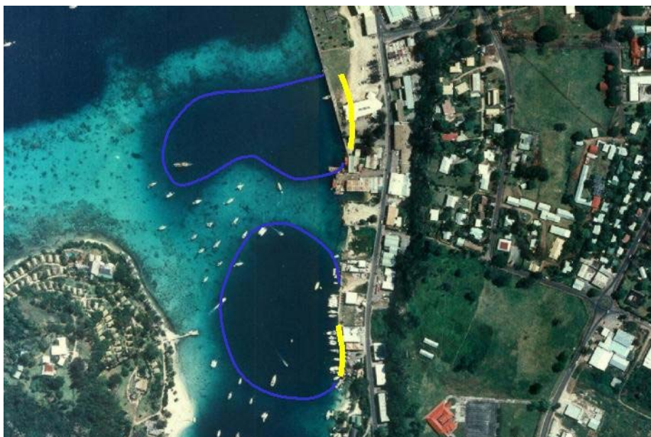
Figure 37: Areas of damaging settlement (yellow lines) during the 2002 earthquake in reclamations over deep harbour areas (dark blue lines)
