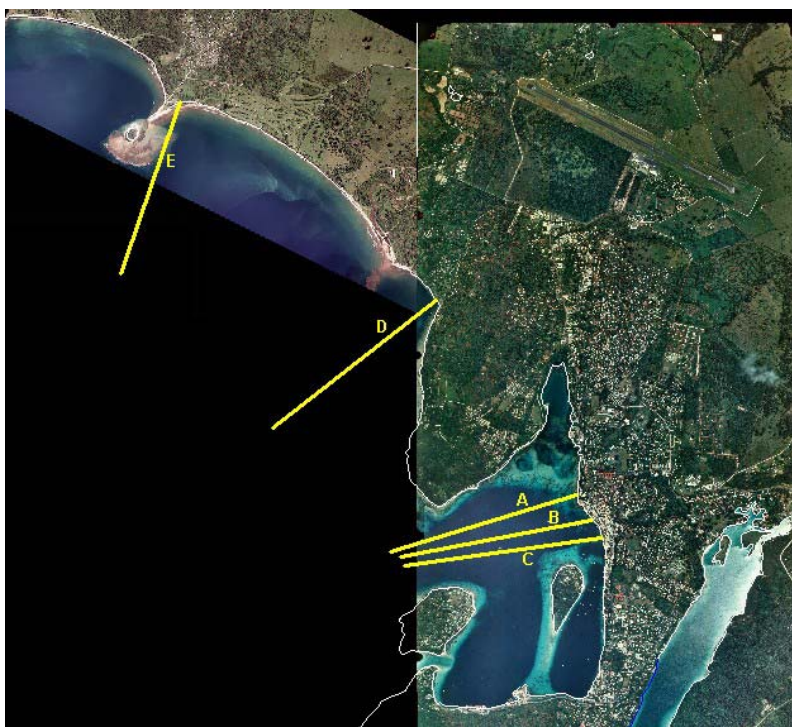
Figure 18: Sections A-E used for calculating storm wave heights, Port Vila Harbour-Mele Bay
