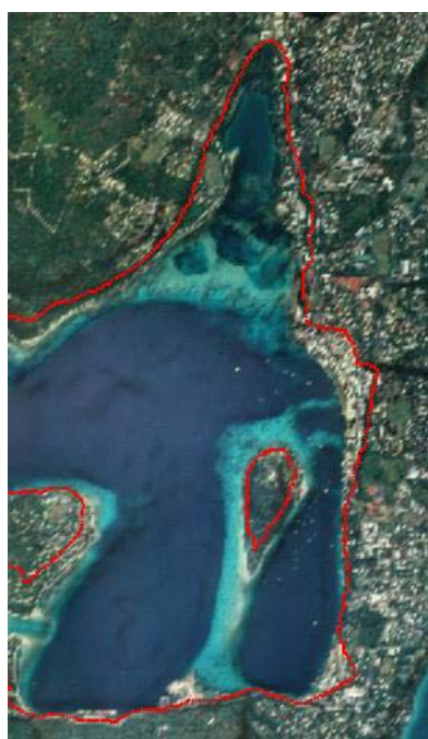
Figure 43: Maximum computed tsunami inundation line
