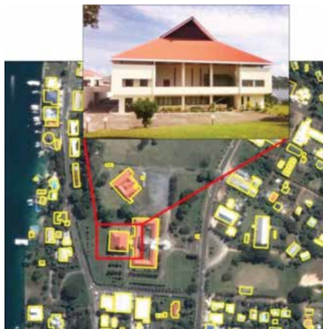
FIGURE 10. Digitized roof footprints of building in Port Vila, VU, and a picture of a building taken by the field inspectors
