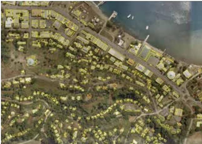
FIGURE 4. High-resolution satellite imagery and digitized building footprints (yellow outlines) in Honiara (SB)
