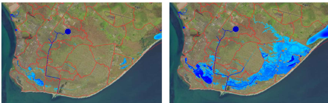
Figure 25 – (left) flood map of a 1-in-5 year storm surge. No flooding occurs, except for the banks of the Rio Chiveve, which causes no damage. (right) flood map of a 1-in-50 year storm surge. Here, clearly the eastern part of the coastal protection is overtopped. Water accumulates in the lower parts of the coastal parts of town.
