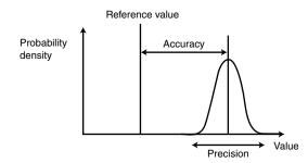
Precision (stability) of a measure vs. accuracy (conformity to actual value).
