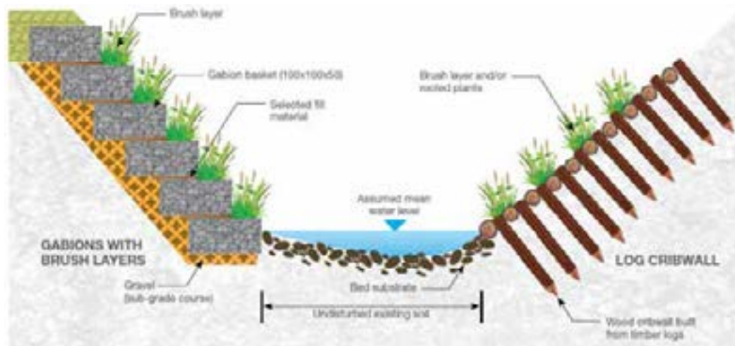
FIGURE A.4. A BIOENGINEERING STABILIZATION TECHNIQUE APPLIED IN THE KALLANG RIVER IN SINGAPORE
